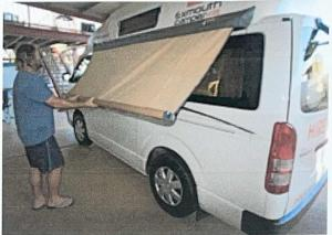
**STEP 3:** Have one person holding middle of leading edge, over head, while the other begins to swing, twist, extend & lock vertical poles into a height position.
